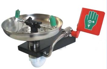
Open 316L stainless steel bowl, wall-mounted emergency eye/face wash featuring twin spray nozzles protected by dust covers. When activated via the push plate, the water jets lift off the dust covers. The eye wash diffusers are fitted with fine mesh strainers and individual flow controllers designed to give a gentle flow of aerated water.
