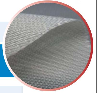
Fiber Type: Finish/Coating: **E-Glass - Thermoglass** Weave-lock (Acrylic Resin)
